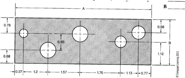
4.) Use the CAD drawing of the plate below to determine dimensions A and B.
