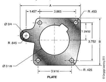
5.) Calculate the perimeter of the symmetrical shim below.
