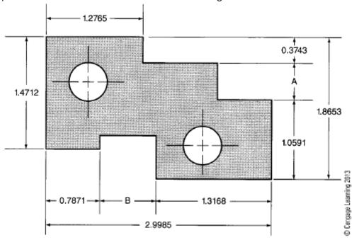
2.) Determine the outside and inside perimeters of the CAD drawing below.
