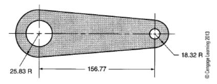
9.) Calculate the overall length on this CAD drawing of a sliding lever.
